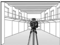
Reference for window installation
